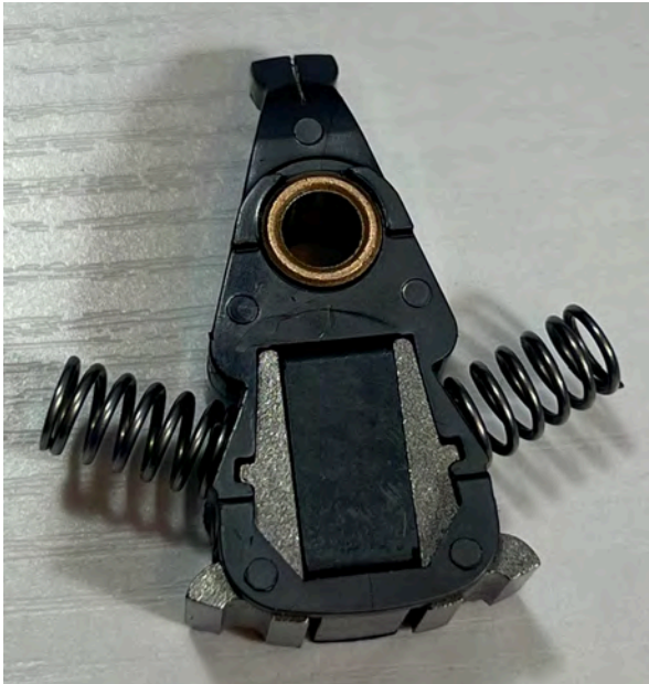
Figure 11 Drive Lever Subassembly
