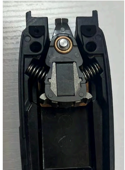
Figure 12 Drive Lever Sub-assembly
